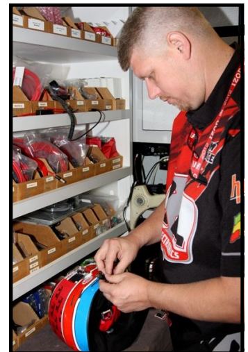
Davin Vesey finishes the installation of a microphone and wiring harness in Mason's helmet. Photo credit: Brad Bernstein
